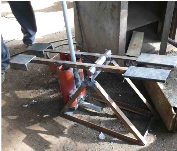
Product development: The mobile treadle pump will be introduced in the next dry season. Its advantage is that it can be used flexibly on more than one well. It further corrects the weakness of the fixed only treadle pump, namely the breaking of the wood pedals. The production costs of the mobile treadle pump are estimated at GHS 109 (as of March 2011).
