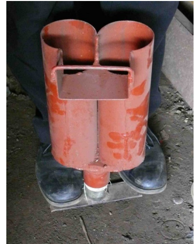
iDE Ghana staff controls quality in terms of leakage and cylinder uniformity.
