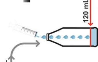
2 The volume of the brine must represent 1/13 of the total volume for electrolysis.
