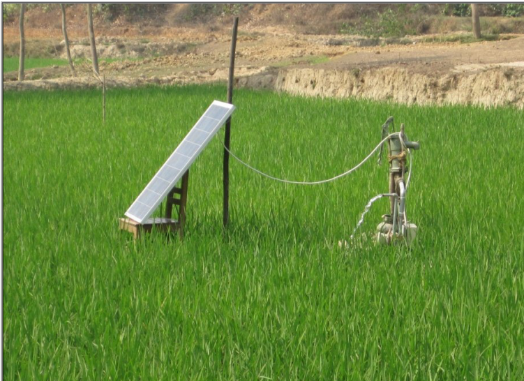
Micro solar water pump installed in rice field
