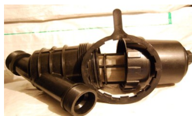
Picture 3: Indian made plastic filter, flow rate 5m 3 /hour
