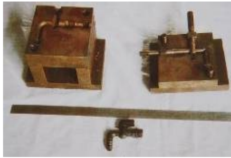
Picture 1: Indian made single cavity mould for plastic valve
