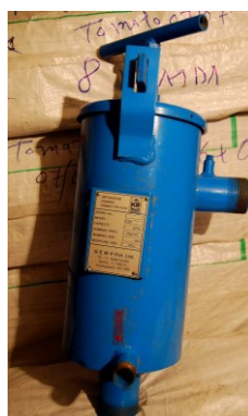
Picture 4: Indian made metal filter, flow rate 20m 3 /hour
