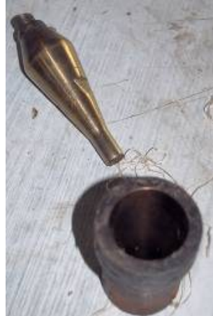
Picture 3: Indian made dye and sizer unit for 4mm diameter pipes with 1mm wall thickness
