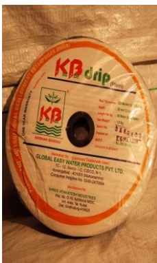
Picture 7: Indian LLDPE laterals, 250 micron, and plain, delivered as 1 kg rolls, ~ 80 m
