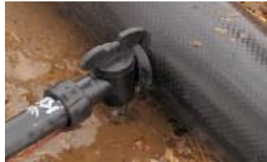
Picture 13: Take off valve fixed to the sub main by a rubber grommet
