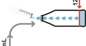
2 The volume of the brine must represent 1/13 of the total volume for electrolysis.
