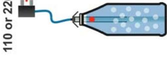
5 Plug in the **Mini-WATA** power supply (5) (110 or 220 V). Bubbles should immediately be seen forming in the bottle. Wait 15 hours to produce 1.5 L of concentrated chlorine (6 g/litre or 6000 ppm)
