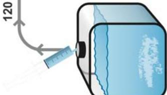
1 Using the large (50 mL) syringe, put 120 ml of saturated brine (1) into a 1.5L bottle (2).
