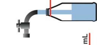
3 Top up the bottle with water (3) until full and immerse the **Mini-WATA** in the salt solution. The liquid level must be above the lateral holes in the tube (4).
