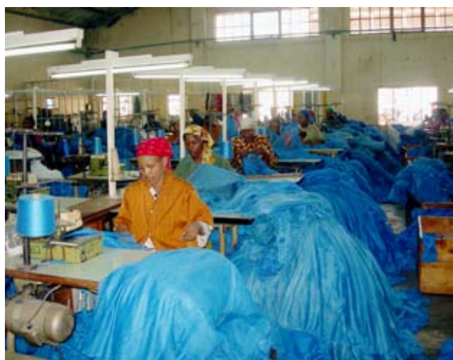
Making bednets is labour-intensive, with several steps of weaving, sewing and finishing before the nets are ready. Pictures from the Sunflag factory in Arusha.
