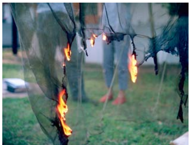
Many tests were necessary, for example to test whether bed nets are dangerous when catching fire.
