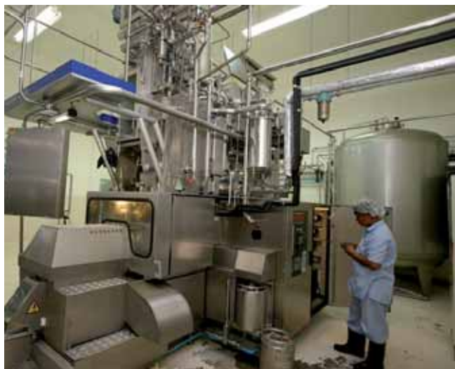
The "core" of the plant is this modern tetra pak packaging machine
