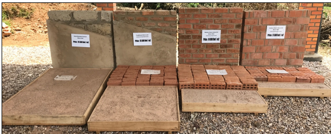
Figure 12: Prices and resources needed for different types of walls with the same size (traditional bricks are left and modern bricks are on the right side)
